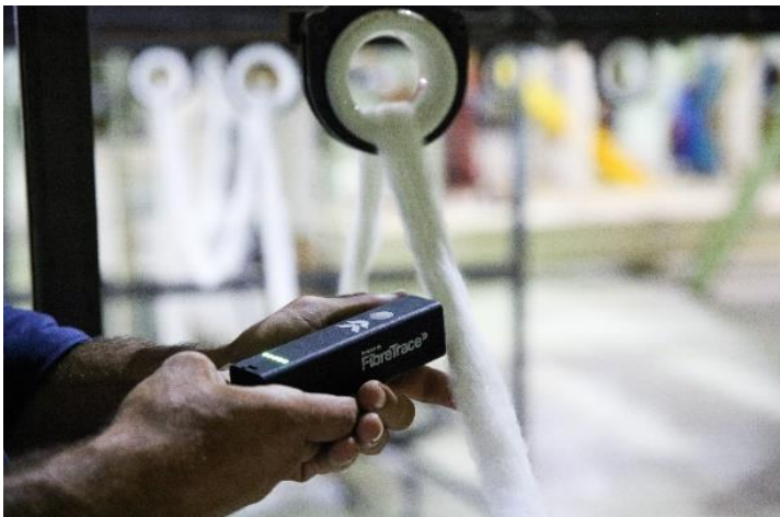
Source: The FibreTrace® scanner for the detection of verified material (FibreTrace®, photo: Olivia Repaci)
