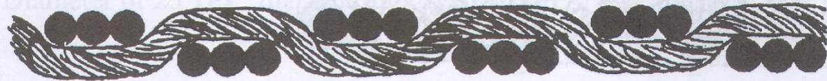
2.9 In 3/3 twill only six interlacings provides space for 18 threads in the space of one inch.
