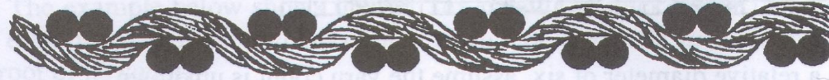
2.8 In 2/2 twill there is sufficient space to allow 16 threads in the space of one inch.
