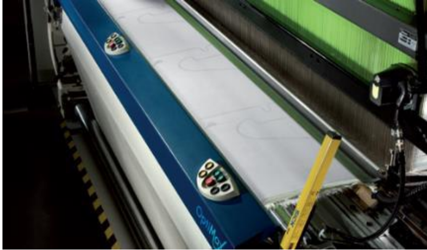
Airbag , including one-piece-woven cushions
