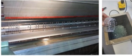
Warp knitting process for manufacture the grid-like shapeable structures Formwork for the concreting process
